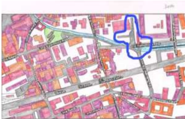
Figure 8. The roads which are separated by the river could be connected by a bridge and a small road could be built to allow access to the houses and flats which flank the present road
